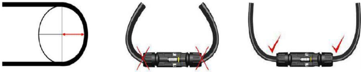
FIGURE 21 MINIMUM BENDING RADIUS OF THE CABLE
